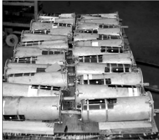
PTP-4 TYPE A VARIABLE SPRINGS WITH A DOWNWARD TRAVEL OF 1.375"
