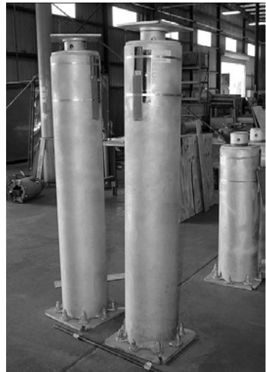
PTP-6 F-TYPE VARIABLE SPRING SUPPORTS
