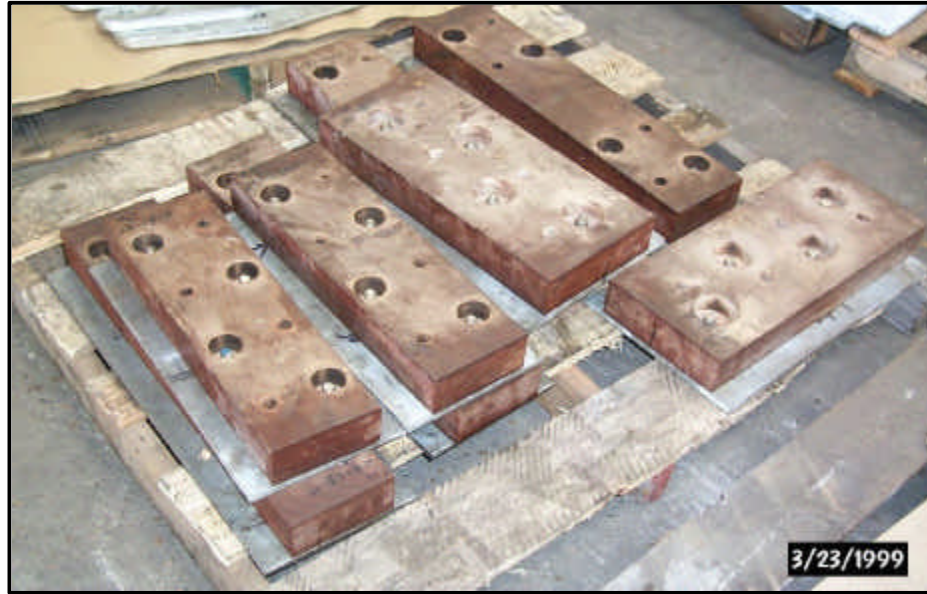
Phenonic Blocks used for F-2 and F-3 Cryogenic Supports
