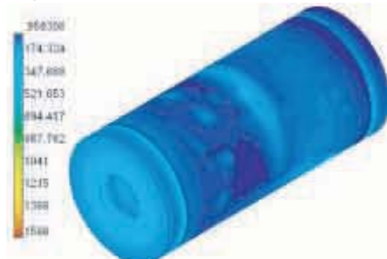
[Figure A11: S stresses in 6 inch insulation]
