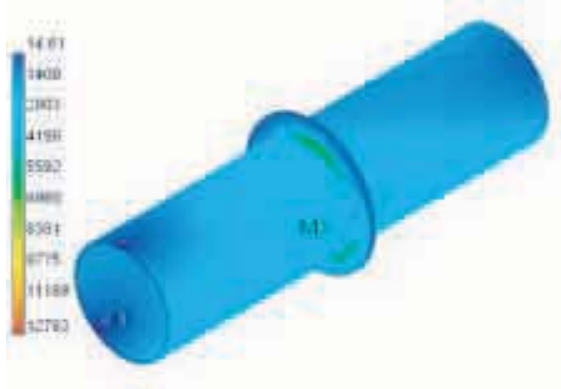
[Figure A4: Stresses in ringpipe]
