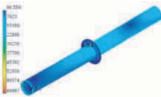
[Figure A10: Stresses in pipe and ring]
