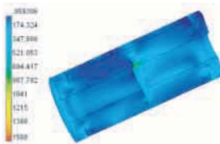
[Figure A12: Stresses on insulation section]
