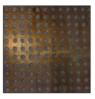
The Bronzphite and its cylindrical grooves filled with the graphite.
