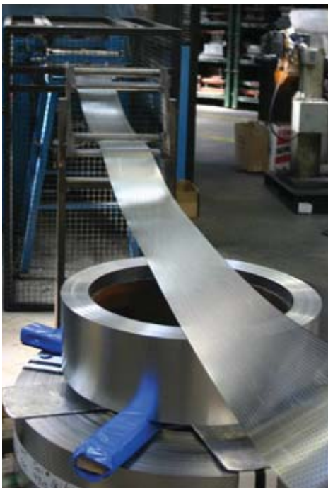
Figure 3 - Picture of Thin Gauge Steel Better Suited to Painting
